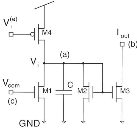
Fig. 2. The E-cell circuit composed of four MOS transistors. Each external input is given to the circuit as the gate voltage  $V_i^{(e)}$ . The E-cell circuits are connected with the H-cell circuit through the terminals (b) and (c).
