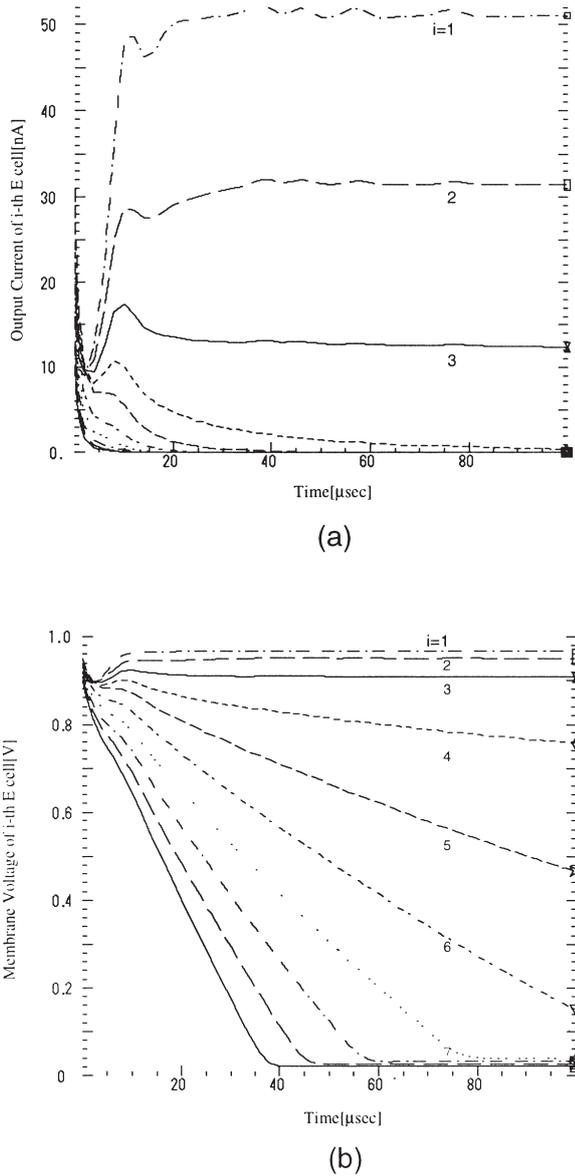
Fig. 4. The dynamic behavior of the circuit model showing the WSA solution with three winners. The time courses of the output currents  $I_i^{M_2}$  and the membrane voltages  $V_i$  at the node of the E cells are presented in (a) and (b), respectively.
